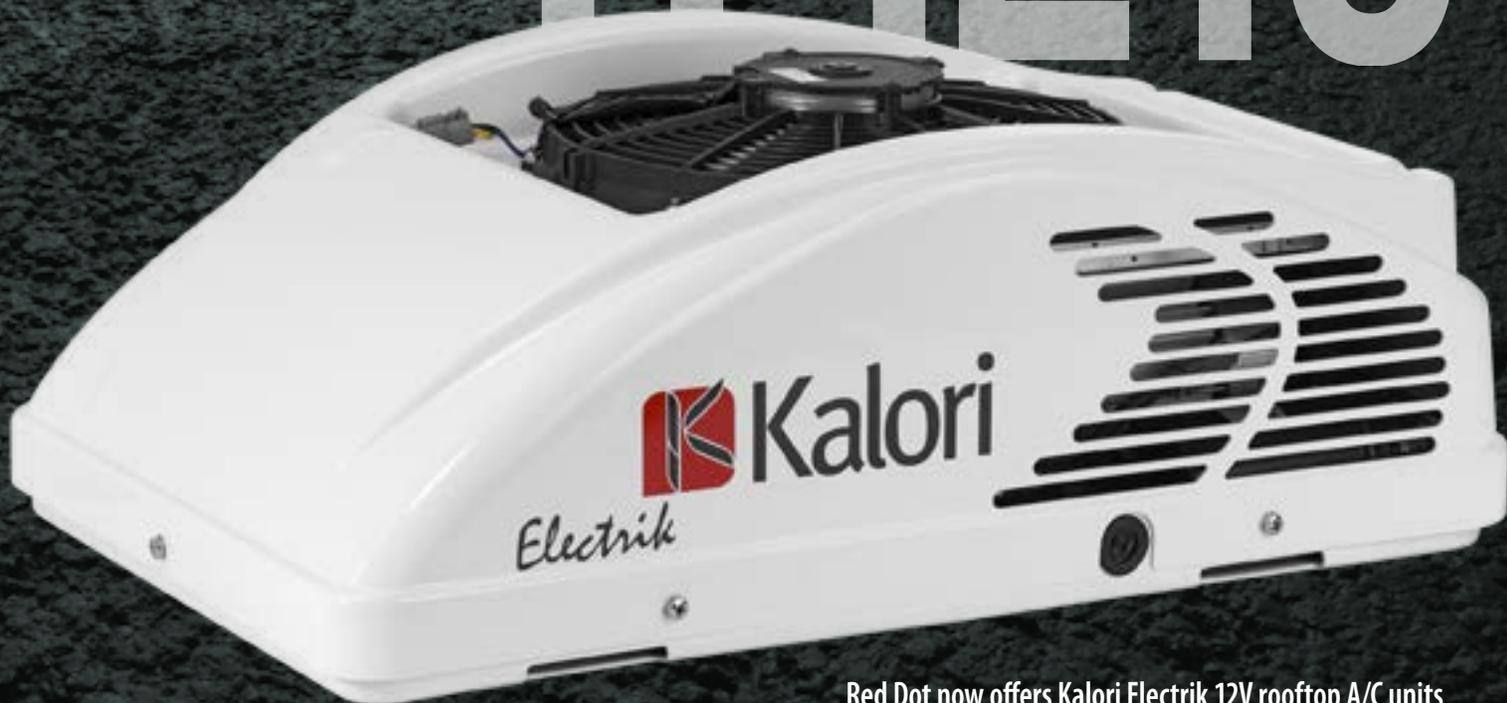
Red Dot now offers Kalori Elektrik 12V rooftop A/C units for on-road applications. With three blower speeds and five rotating air diffusers, the unit delivers cooling performance in the 11,900 BTU/ hr range. Note that it also draws up to 80 amps; the unit is designed to be used with the engine running and is not an engine-off system for heavy-duty cabs or sleepers.
